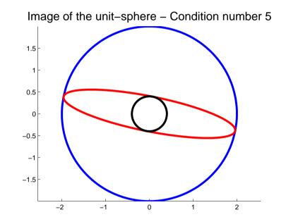
The condition number can be seens as measuring the distortion of the unit sphere under the mapping of A. The higher the condition number the more elongated become the level sets of the second-order approximation.
